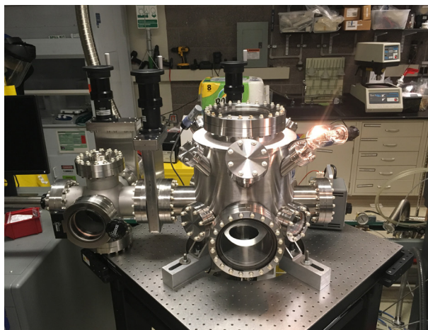
▲ Figure 2: The SAFEM UHV chamber and subnano positioner stage.
