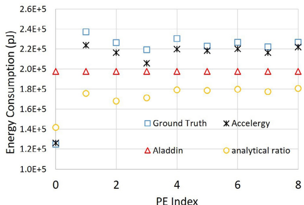
▲ Figure 2: Energy estimation comparison on the energy breakdown across the processing engines (PEs); in Eyeriss PE array (only selected PE are shown).
