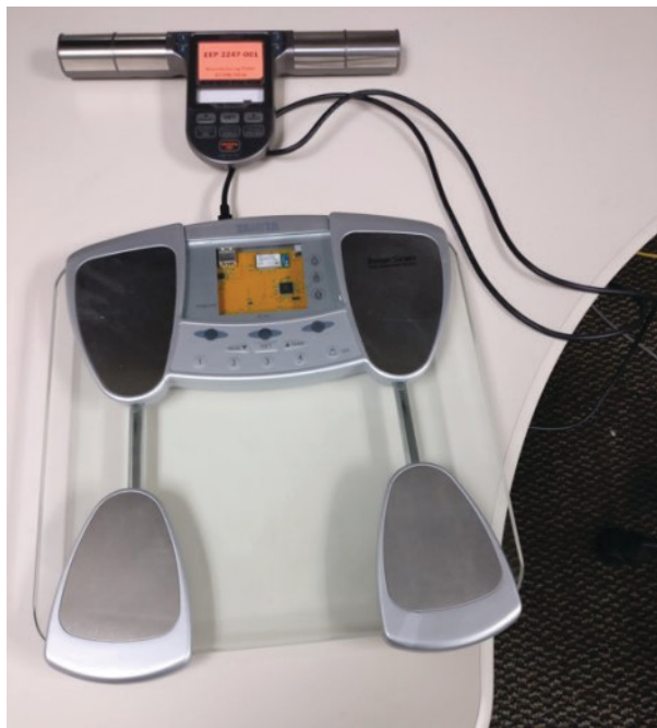
▲ Figure 1: The device shown here is used to generate the BCG waveform. The scale contains the force sensor and the handlebar uses electrocardiography and is used to help process the BCG signal.
