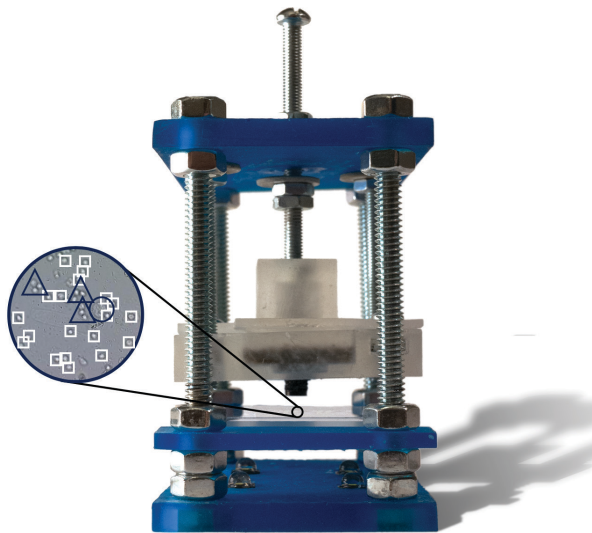
▲ Figure 1: A side-view of the AutoScope system. The cost of the bill-of-materials is $57-$92. The end-to-end resolution is 5.86-8.29 \mu m.
