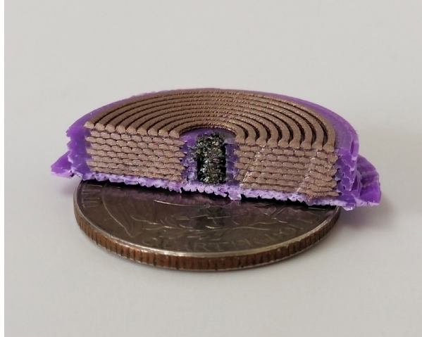
▲ Figure 1: Three-dimensional, monolithically 3D-printed FeSiAl nylon-cored solenoid cut in half, on top of a U.S. quarter.
